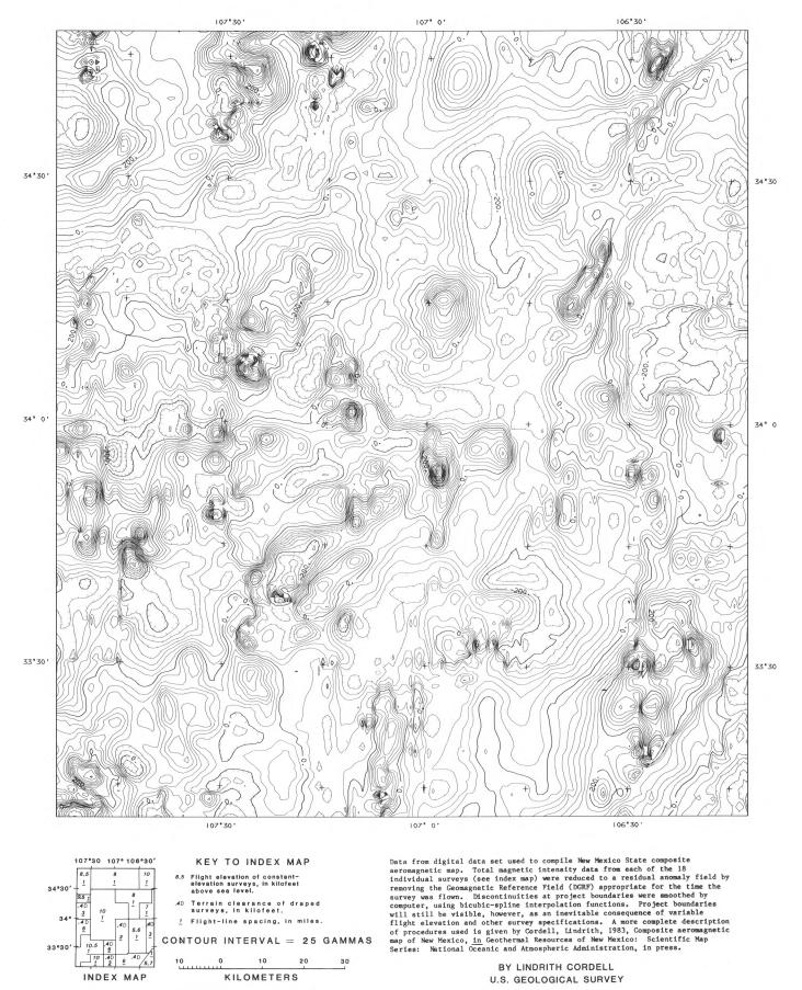
COMPOSITE RESIDUAL TOTAL INTENSITY AEROMAGNETIC MAP OF THE SOCORRO REGION, NEW MEXICO
