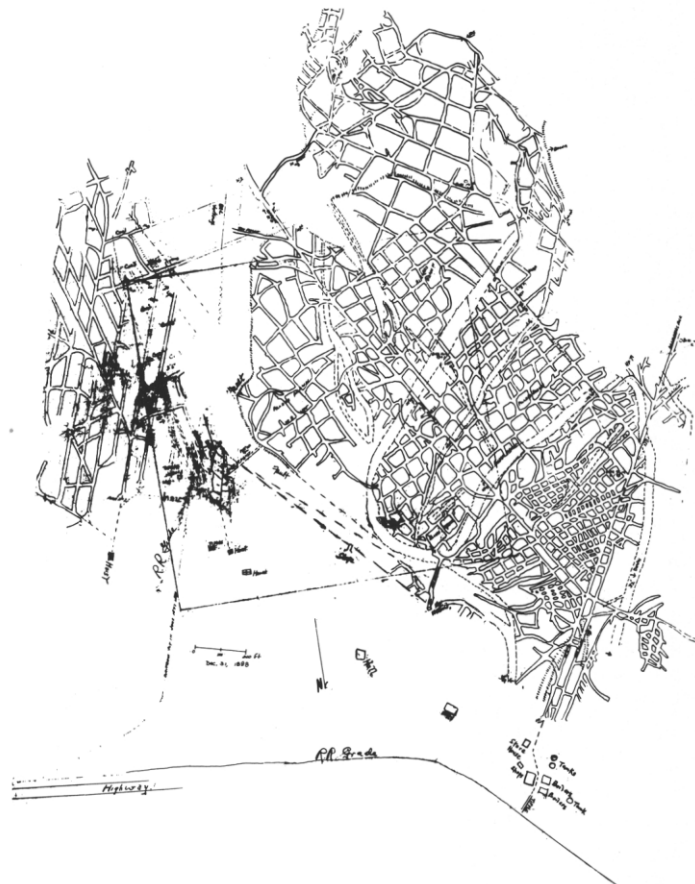
Figure 3. Mine map circa 1888 of the Manila (left) and Santa Fe mines, located at SW 1 / 4 SW 1 / 4 sec. 10, T5S, R2E, showing highly modified room and pillar pattern. All of the dotted and hachured lines are faults.
