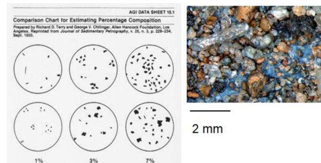
A size comparison chart used for petrography, left, and a view of a composite dump sample, right
