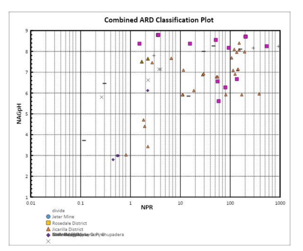
Acid Rock Drainage (ARD) plot of waste rock pile at mines examined during the NMBGMR AML project. The results for the waste rock piles from the Little Davie, Lucky Don, Chupadera, and Jeter uranium mines (Socorro County), St. Anthony uranium mine (Cibola County), Rosedale and Jicarilla gold mines (Socorro and Lincoln Counties) and Silverton gold-silver mines (Colorado) are shown for comparison (unpublished work in progress). Results of these mines will be published in future reports.
