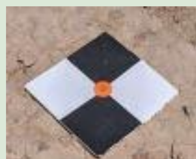
A target used as a ground control point
