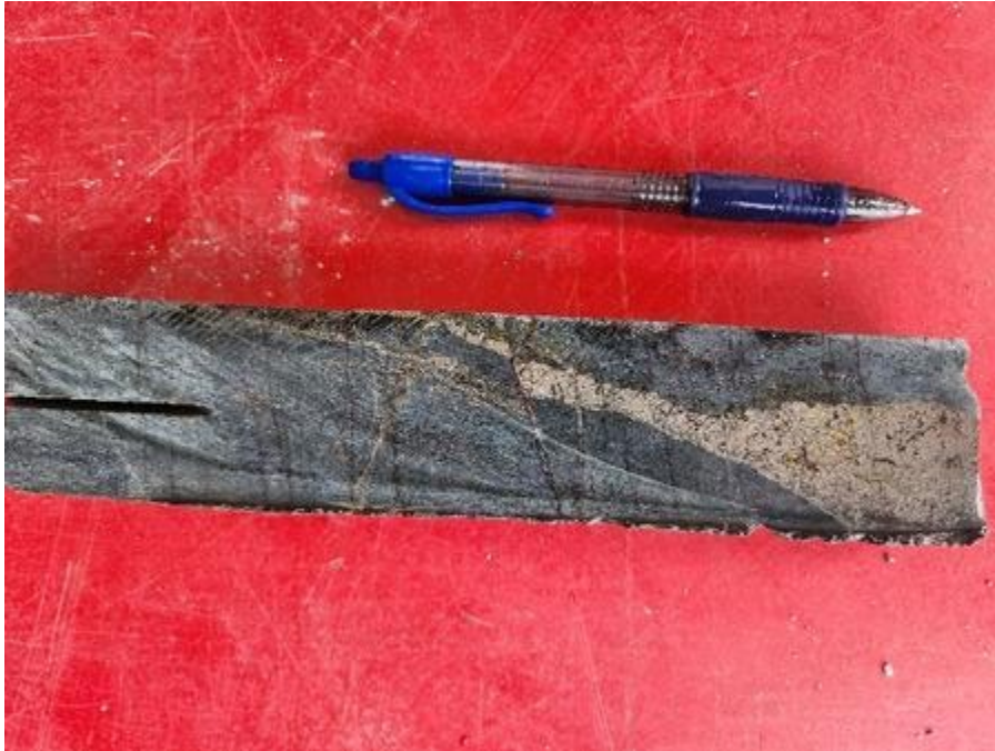
Concentrated vein of Fe-Cu sulfide minerals in rock from Jones Hill Sample 247 (04/18/24). Photo credit: Jennifer Lindline.
