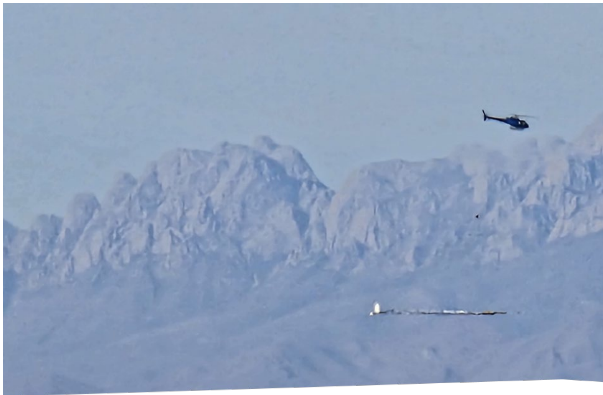
SkyTem's AEM system in the Lower Mesilla Basin.
