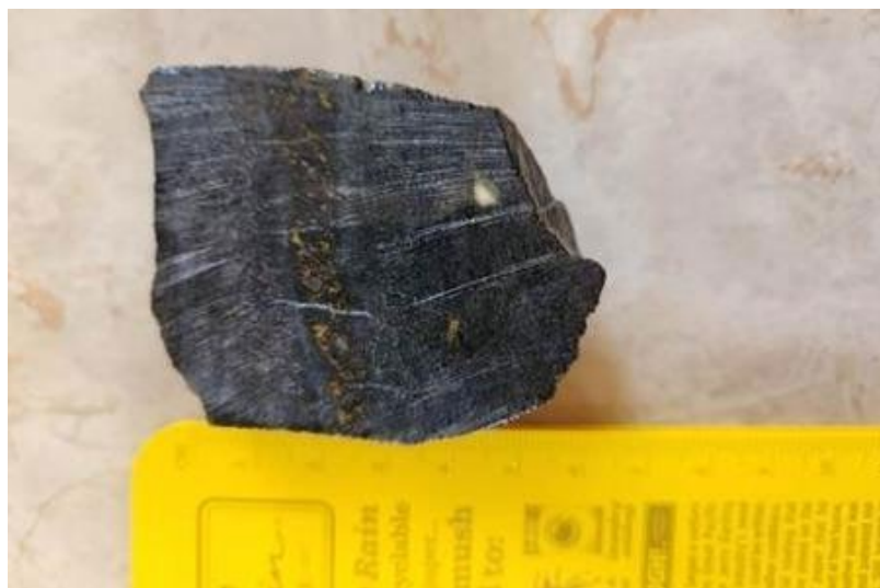
Photo of discreet cubes of pyrite and concentrated vein of Cu-sulfide minerals in rock from Jones Hill Sample 250 (06/13/24). Photo credit: Jennifer Lindline
