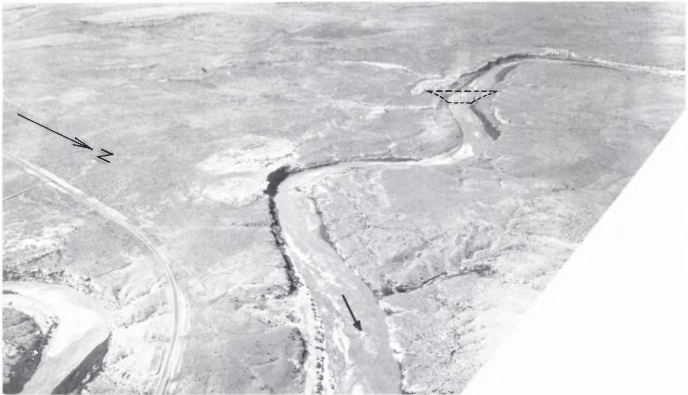
Figure 1. Aerial view southwest from above Logan (up Canadian R.) showing outcrops of Trujillo Formation and Ute dam site (downstream from upper Bend). Light-colored rim of Canadian River at upstream margin of photo is west limb of Ute anticline. Photo by N. S. Long.
