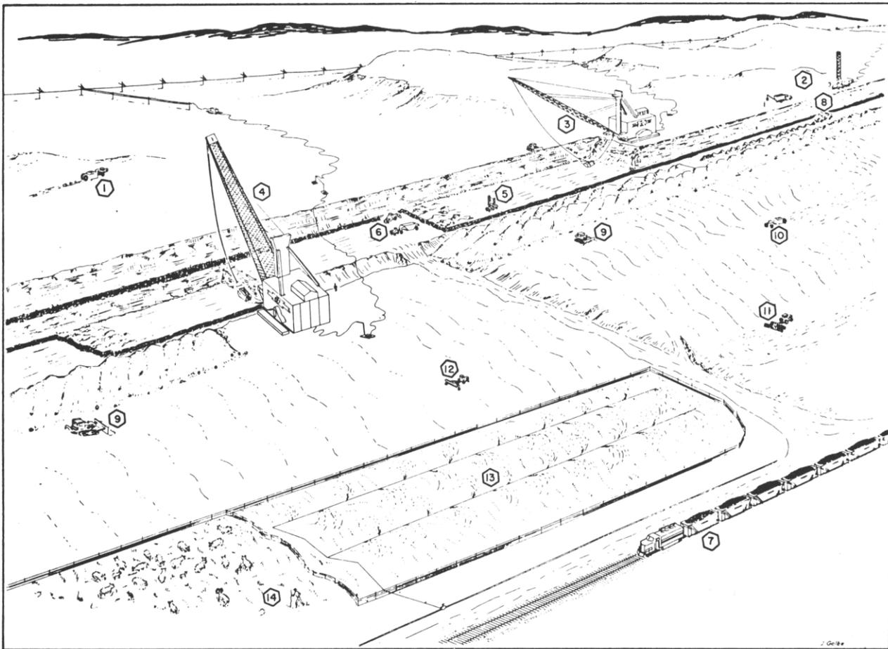
Figure 1. Typical operation at Navajo mine: (1) topsoil investigation; (2) overburden drilling; (3) stripping; (4) dragline operation; (5) coal drilling; (6) coal hauling; (7) transport facilities; (8) stockpiling; (9) ash disposal; (10) grading of spoil piles; (11) erosion control grading; (12) discing and revegetation; (13) sprinkler operation; and (14) completed land restoration.
