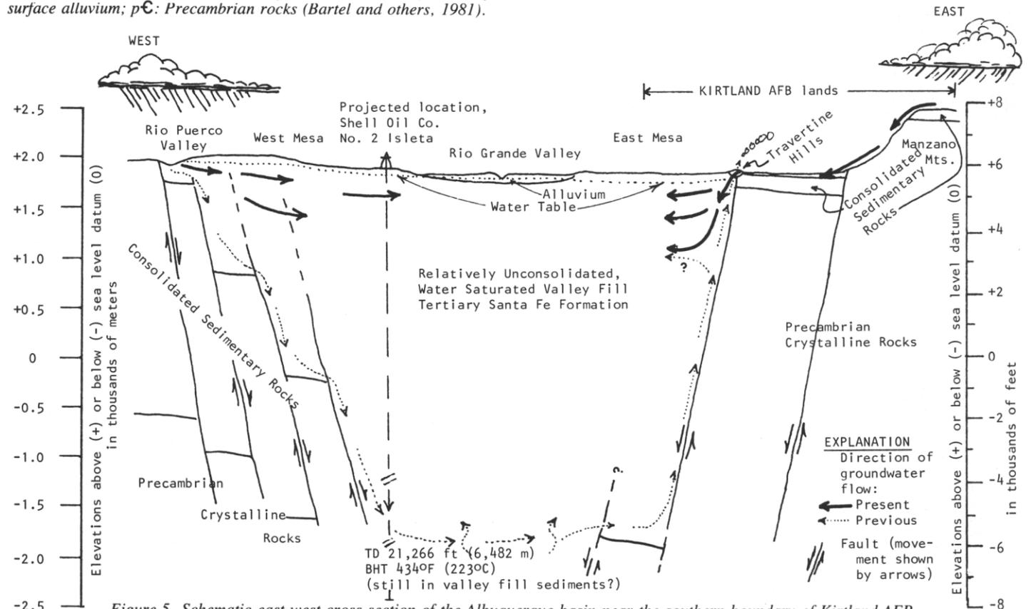
Figure 5. Schematic east-west cross section of the Albuquerque basin near the southern boundary of Kirtland AFB.
