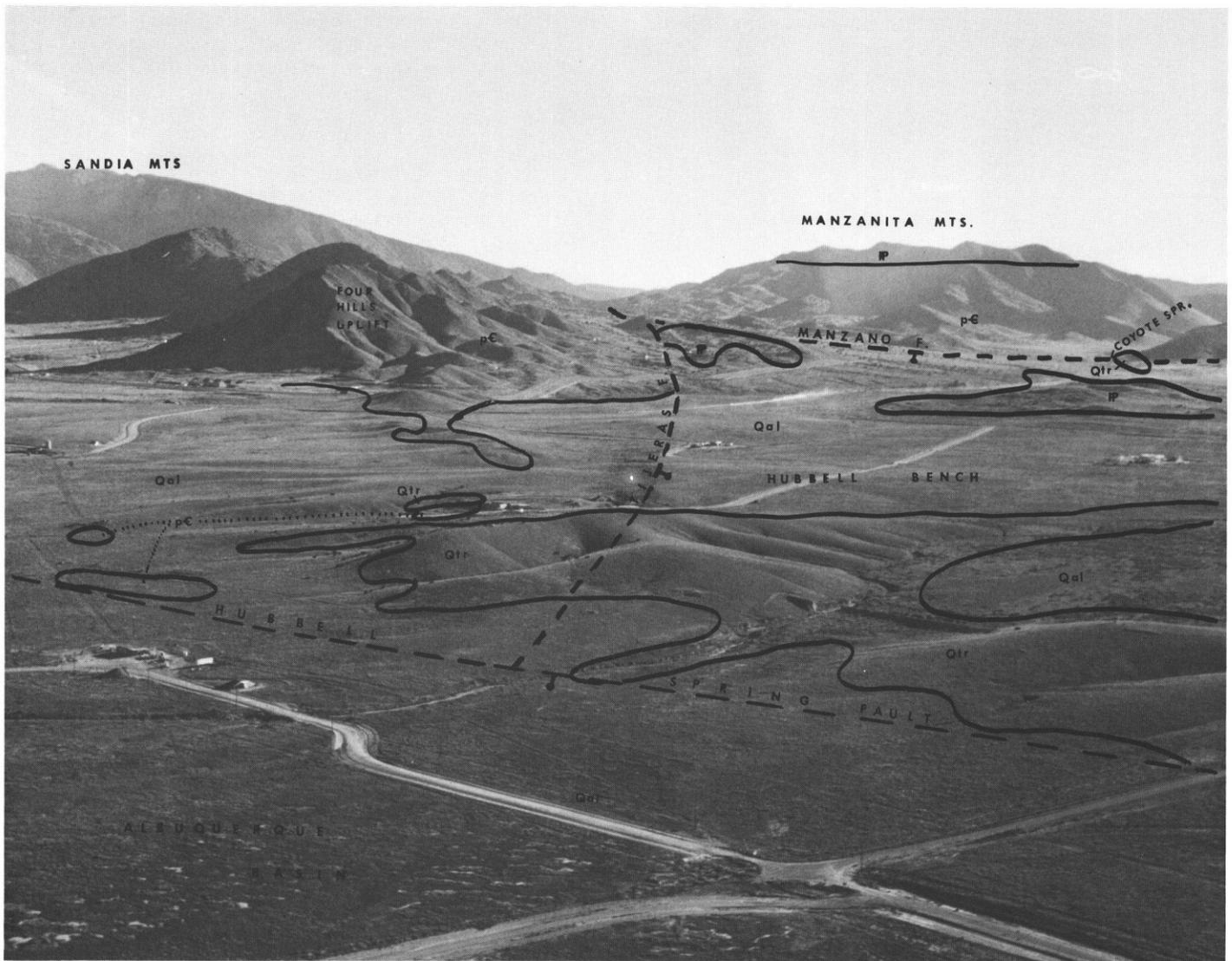
Figure 2. Structural and stratigraphic relationships along the Hubbell Spring fault, Kirtland Air Force Base. Air view from position about 11.2 km (7 mi) south of Eubank and Central intersection in Albuquerque. Qal: Quaternary surface alluvium; Qtr: Quaternary travertine deposits; IP: Pennsylvanian rocks; pC: Precambrian rocks.
