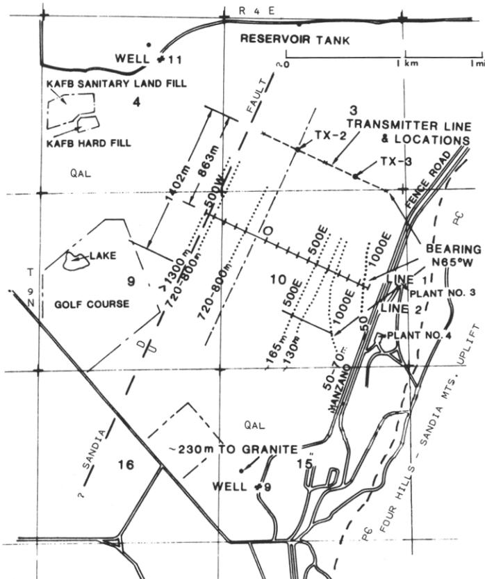
Figure 4. Controlled source audio-magnetotelluric (CSAMT) electromagnetic (EM) geophysical experiment east of Four Hills uplift. Sandia fault identified by long dashed line, downthrown to the northwest. Depth to basement (granite) in meters shown by dotted lines. Qal: Quaternary surface alluvium; pC: Precambrian rocks (Bartel and others, 1981).
