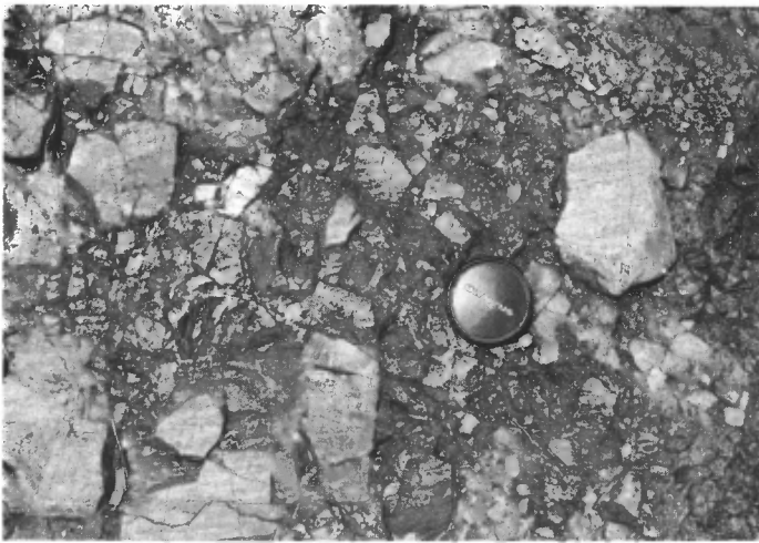
FIGURE 6. Quartzite breccia from the southern metasedimentary terrain. Angular, lined quartzite clasts of variable size are set in a medium-grained quartzite matrix. Lens cap is 5 mm across.
