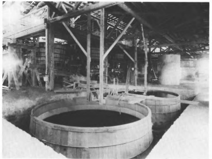
FIGURE 6—Vanadinite concentrates were leached with sulfuric acid in the upper tanks; the vanadium-sulfate solution was then decanted, probably to the holding tanks, foreground, from where it was taken, apparently by hand, to an evaporating furnace followed by calcining to V_2O_5 . Photo courtesy Mrs. Lydia Key, Black Range Museum, Hillsboro.
