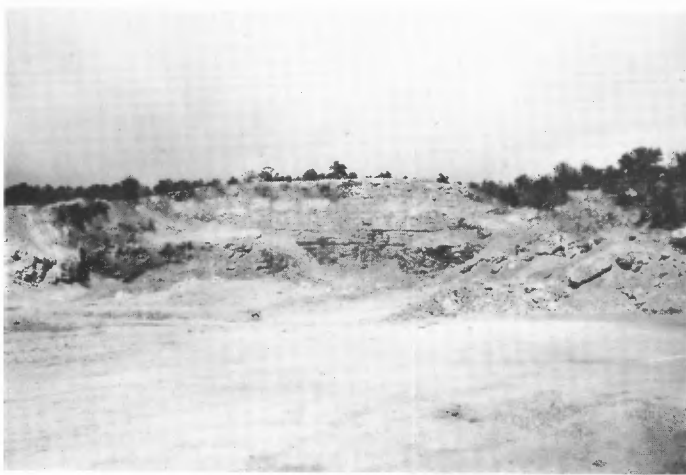
FIGURE 3-64.7g. View to east of aggregate pit developed in San Andres Ls. Near middle is a 15-ft-thick section of mudstone, white Glorieta-type ss and maroon, very fine-grained ss.
