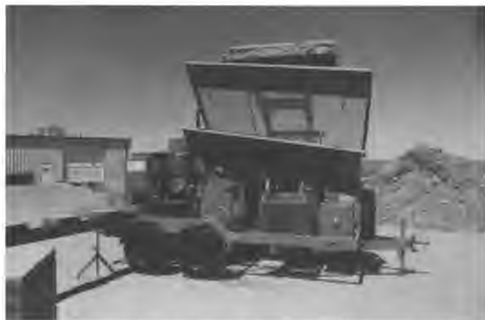
FIGURE 4. Worldwide Adobe, Inc., Goldbrick "5000" pressed-earth block machine at the factory located near Grants, New Mexico.
