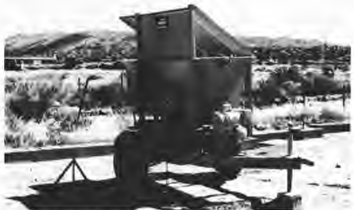
FIGURE 1. Earth Press III pressed-earth block machine on a wall-construction site near Velarde, New Mexico.
