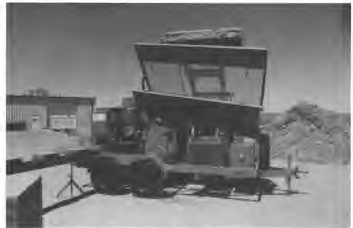
FIGURE 4. Worldwide Adobe, Inc., Goldbrick "5000" pressed-earth block machine at the factory located near Grants, New Mexico.
