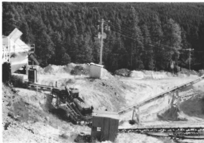
FIGURE 8. View north toward mine in the background. Screening plant and pit partly obscured by stockpiled boulders (left) and crushed ore (right).
