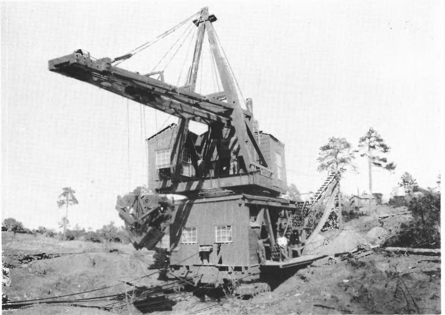
The American Placer Company installed this cantilever-type placer machine and attempted to work the gold placers along Ancho Gulch in the Jicarilla district during 1903-4. Manufactured by W. M. Johnston & Co. of Chicago, the machine was not a dredge, as often stated, because it did not float on water. The machine weighed nearly 200 tons and was doubtless difficult to maneuver. That fact, coupled with too much overburden and too little water, led to its failure. Photo by Fayette A. Jones, 1904; courtesy of Museum of New Mexico.
