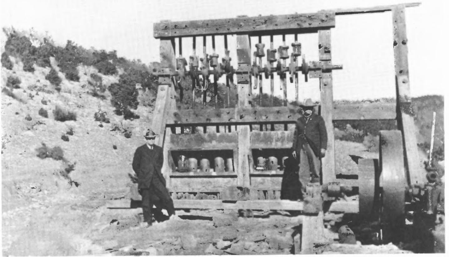
The historic Glass stamp mill was the first to operate in the White Oaks district. Named for Professor Glass, this 10-stamp mill first saw service reducing gold ore at the Rita mine beginning in 1883. Later it was leased briefly by the Old Abe Company. Thereafter it moved to the southeast side of town and stored on the Sam Wells ranch where it was photographed in January 1918. New Mexico Bureau of Mines collection No. 1665, courtesy of Richard H. Jahns and John Kelt.
