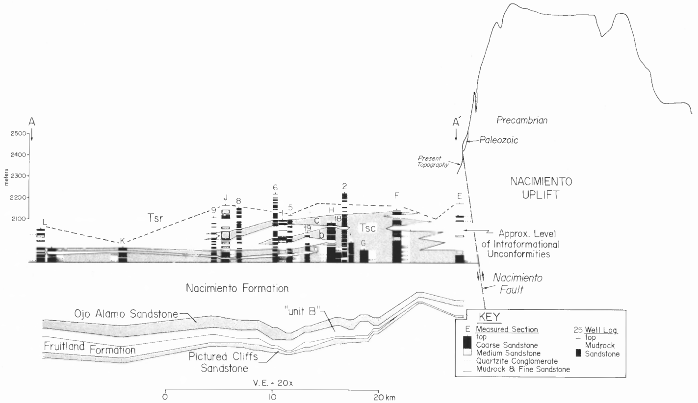
FIGURE 8. Stratigraphic east-west cross section of the upper Nacimiento Formation and lower San Jose Formation near the north end of the Nacimiento uplift. Paleoflow toward the south is inferred by paleocurrent measurements made in outcrops northeast and south of the cross section. The vertical stacking of sandstones in the Nacimiento and San Jose Formations indicates that channel belts persisted in locations parallel to the Nacimiento uplift.
