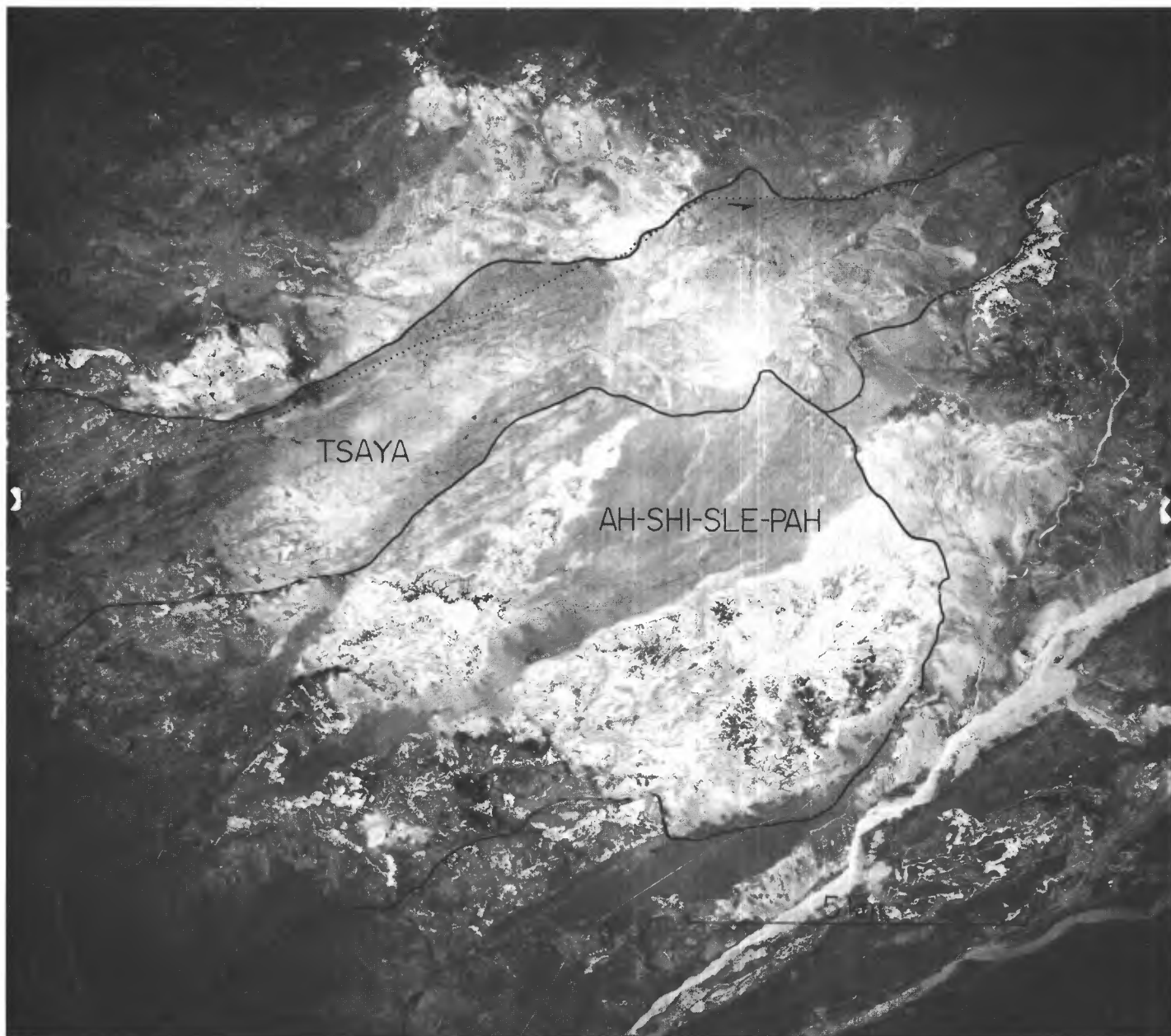
FIGURE 3. Aerial photograph of part of the Tsaya and Ah-shi-sle-pah drainage basins. Alluvial surfaces appear as uniform gray tones; local mottling on these surfaces are sand dunes and blowouts. Note the extensive badland development in the Ah-shi-sle-pah basin, compared to the Tsaya basin. The field trip route is shown by a dotted line and arrows.
