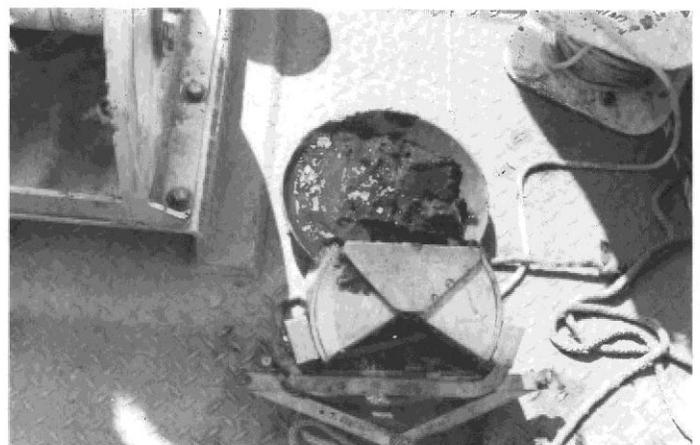
FIGURE 4. Bottom-grab sampler used to collect lake sediments for this study.
