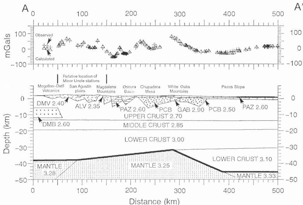
FIGURE 5. Free air gravity model across New Mexico (A-A', Fig. 1). This model is constrained by deep petroleum exploration wells and the results of seismic refraction modeling of Roberts et al. (1991), Sinno et al. (1986), and Olsen et al. (1979). MDV - Mogollon-Datil volcanics, MDB - Mogollon-Datil batholith, ALV - Alluvium, PAZ - Paleozoic, PCB - Possible Precambrian or Paleozoic basin, GAB - Gabbroic intrusion.
