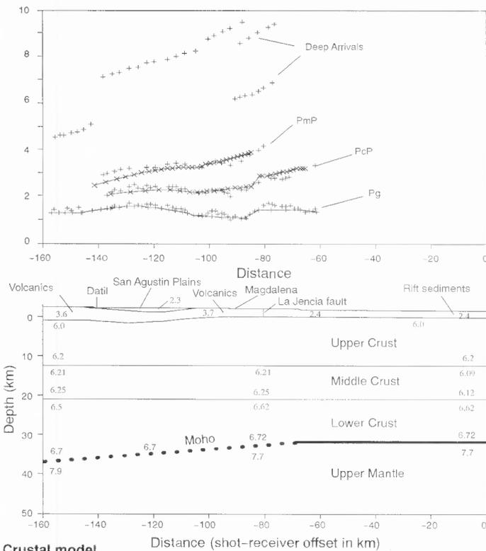
FIGURE 4. Picked arrival times (from Fig. 2) and preliminary earth model derived from ray tracing the Minor Uncle seismic data. Numbers indicate P-wave velocities in km/s.
