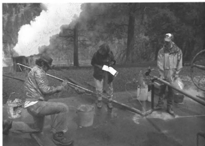
FIGURE 2.12. Sampling operations at VC-2B, May 11, 1992; first mini-separator (by standing man on right) is connected to left side of flow line that runs between well head (behind photographer) and weirbox (steaming in background). Mini-separator is adjusted to separate high-temperature fluid into vapor and liquid components. Sampling line and condensers (in the bucket) are connected to steam-side of separator. Man kneeling on left is collecting a gas sample.
