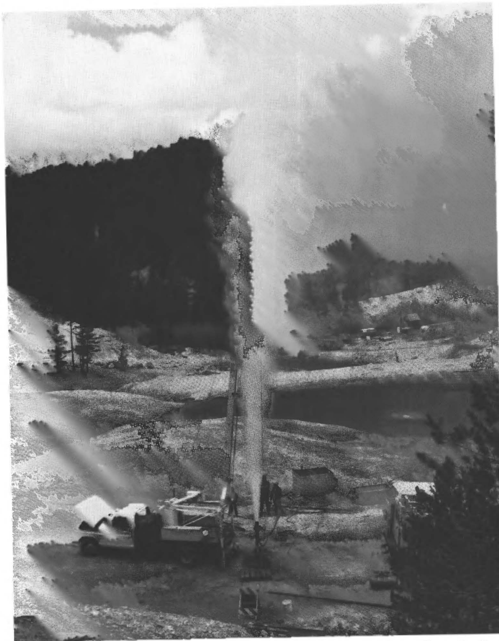
FIGURE 2.14. Photo of VC-2A erupting flashed reservoir fluid from a depth of about 1,600 ft on May 1, 1987, while Lisa Shevenell and landowner John Corbin gaze in awe. Reservoir temperature at this depth is 210°C. The alkaline chloride reservoir fluid has dramatically different chemistry than the acid-sulfate springs at the surface.
