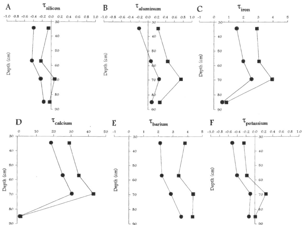
FIGURE 4.  $\tau$  diagrams for the study soil. A, Silicon; B, Aluminum; C, Iron; D, Calcium; E, Barium; F, Potassium. Circles represent calculations with no correction for dust influx. Squares represent calculations with correction for dust influx.
