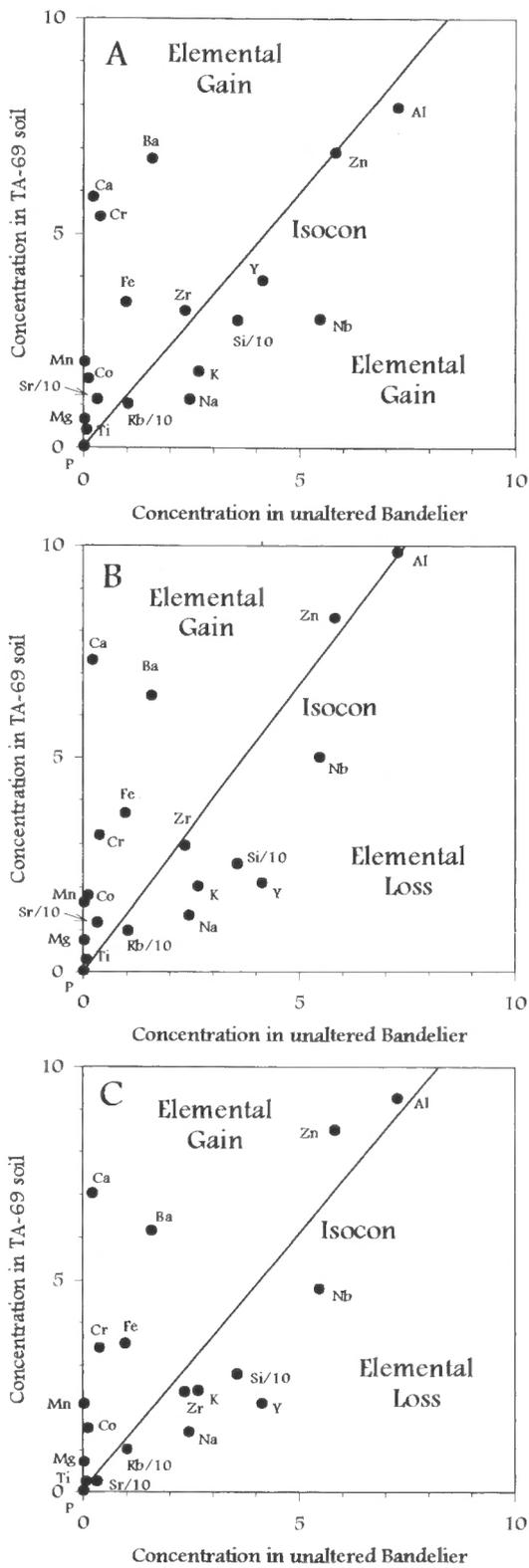
FIGURE 1. Isocon diagrams for the TA-69 study soil. A, 2Bt1b horizon. B, 2Bt2b horizon. C, 2Bt3b horizon. Major and minor elements are in weight percent, trace elements are in parts per million.
