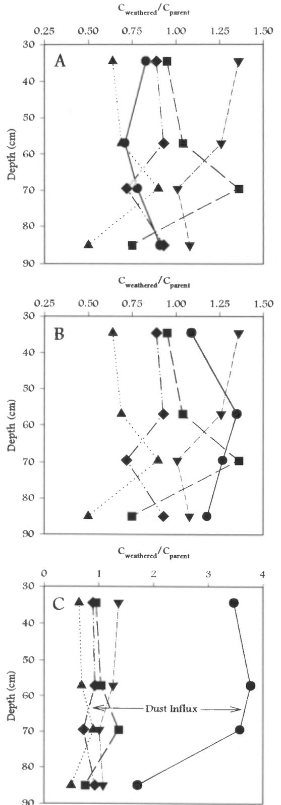
FIGURE 3. Constitutive mass-balance model for A, Silicon; B, Aluminum; C, Iron. Circles, measured ratio; squares, maximum residual enrichment; upward triangles, minimum residual enrichment; downward triangles, uncorrected strain plus residual enrichment; diamonds, dust-corrected strain plus residual enrichment.
