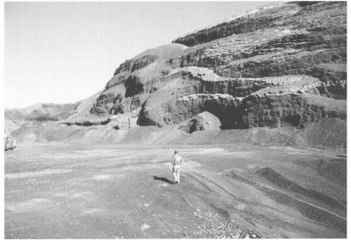
FIGURE 16. The Severo Garza operation on the southwest flank of Guzman Lookout Mountain primarily produces small-size black scoria.
