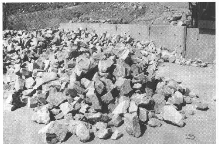
FIGURE 3. Larger blocks of Eocene Vado Andesite ready for shipment from the Vado quarry. The andesite, which produces a tough gray aggregate, is used as large stones to build walls in southern New Mexico and west Texas.
