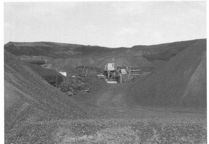
FIGURE 10. Looking west in the Santa Fe Mining Company's Donna Mountain operation, past crushed and screened scoria and over processing equipment toward the crest of the cinder cone.
