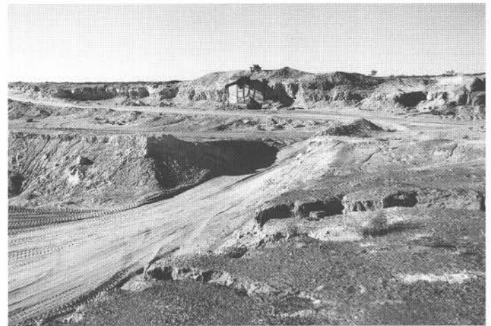
FIGURE 2. La Union fine-grained aggregate pit (BLM) in SE 1/4 sec. 13, T27S, R3E. The small amount of larger-size aggregate is dominated by calcium carbonate-cemented soil derived from the caliche cap.
