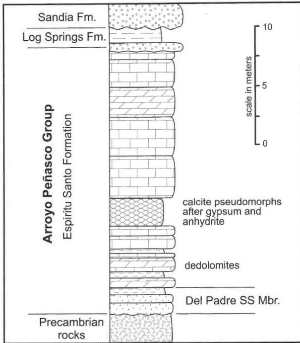
FIGURE 1.5. Measured stratigraphic section of Mississippian strata at Placitas (from Armstrong et al., 1979). Although measured about 3 mi. northeast of Stop 1, the Mississippian section at Stop 1 is essentially the same as shown here.
