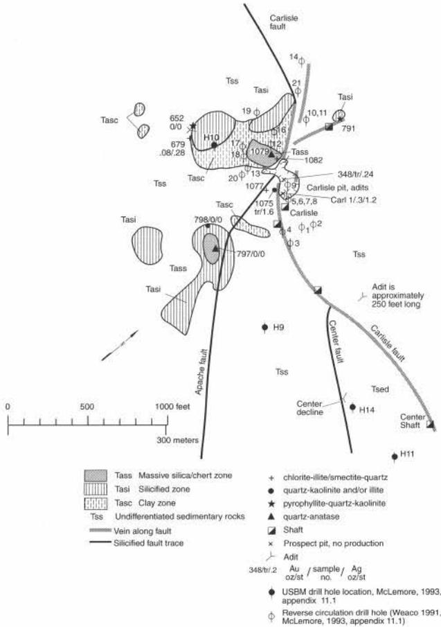
FIGURE S.2.11. Geologic and alteration map of the Carlisle mine.
