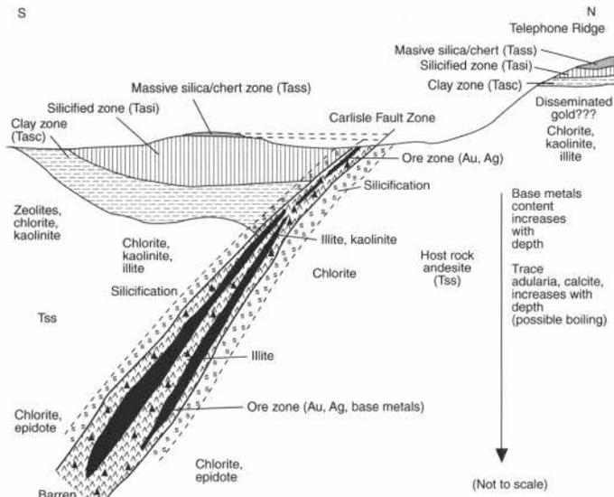
FIGURE S.2.14. Relationship between alteration and vein deposits along the Carlisle fault.
