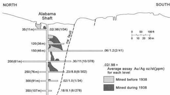
FIGURE S.2.6. Longitudinal section of the Alabama mine (F. W. Smith, unpubl. report, 1910). Does not show mining in 1950 and 1951.
