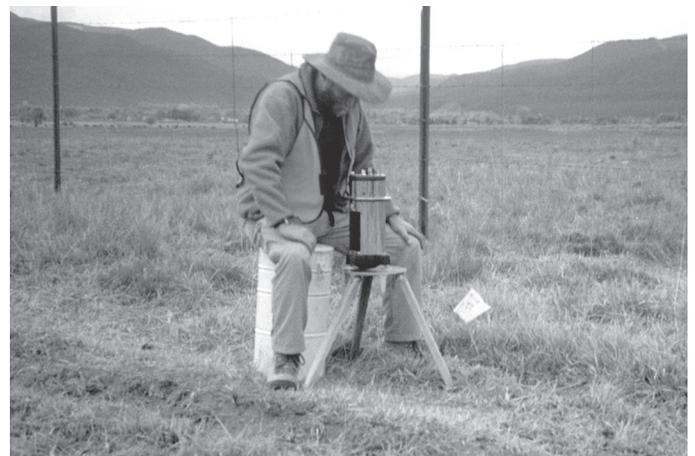
FIGURE 2.19. This area was the focus of a detailed gravity survey in 2001 by the New Mexico Bureau of Geology and Mineral Resources. The survey consisted of 21 separate traverses with 50 m and 100 m station spacing, for a total of 66 km of survey lines.
