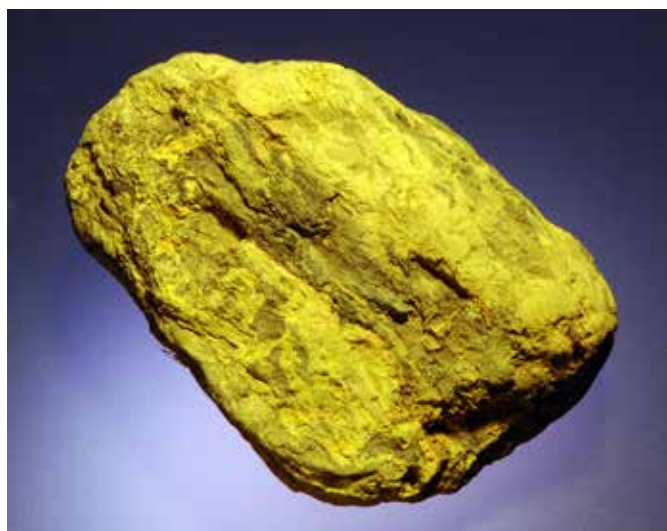
Carnotite, K_2(UO_2)_2V_2O_8 \cdot 3H_2O , on sandstone Specimen is 6 cm long. NMBGMR Museum No. 12690, Carrizo Mountain, San Juan County, NM.
