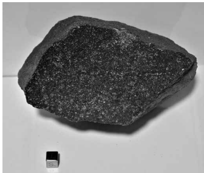
FIGURE 3. Uranium minerals with dark humate in Jurassic sandstone from Grants Mining District (1 cm cube for scale).
