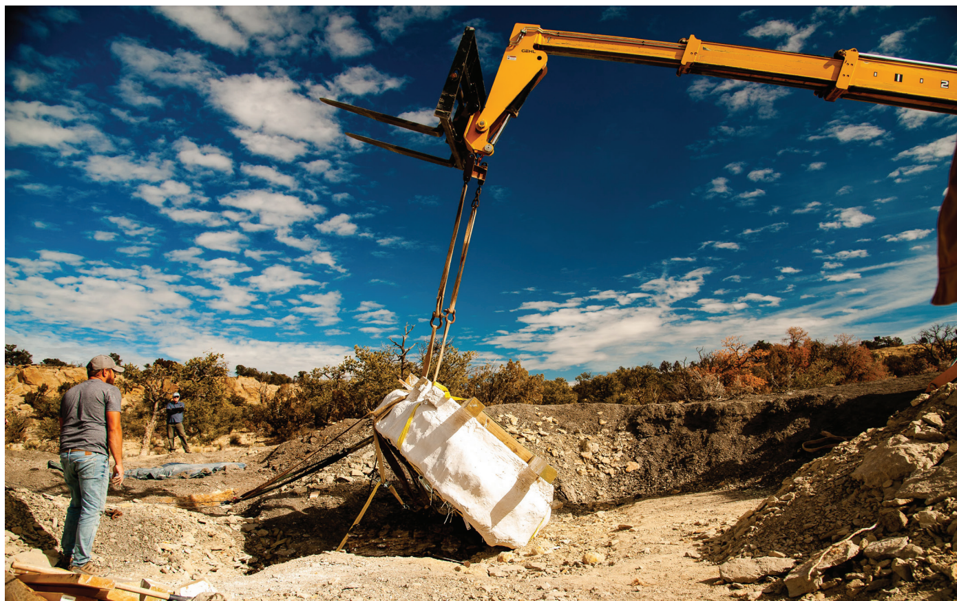
Figure 7. Initial unsuccessful lift attempt with telescopic handler boom arm fully extended.
